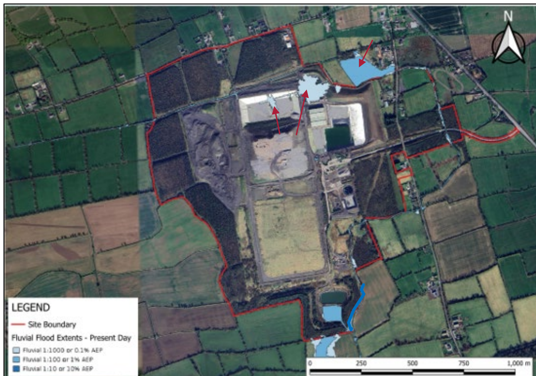
Figure 1: Flood Zone Extents – Present Day Scenario (Source: Flood Risk Assessment submitted in the original application.)
